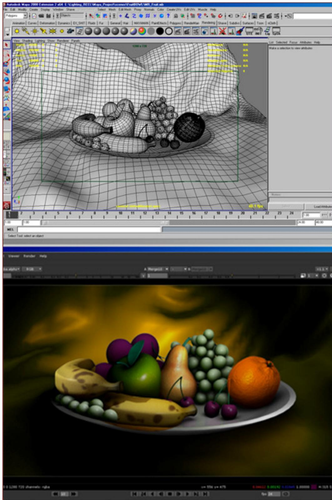
Task of a render engine, Transition between 3D application (top) and image (bottom).
