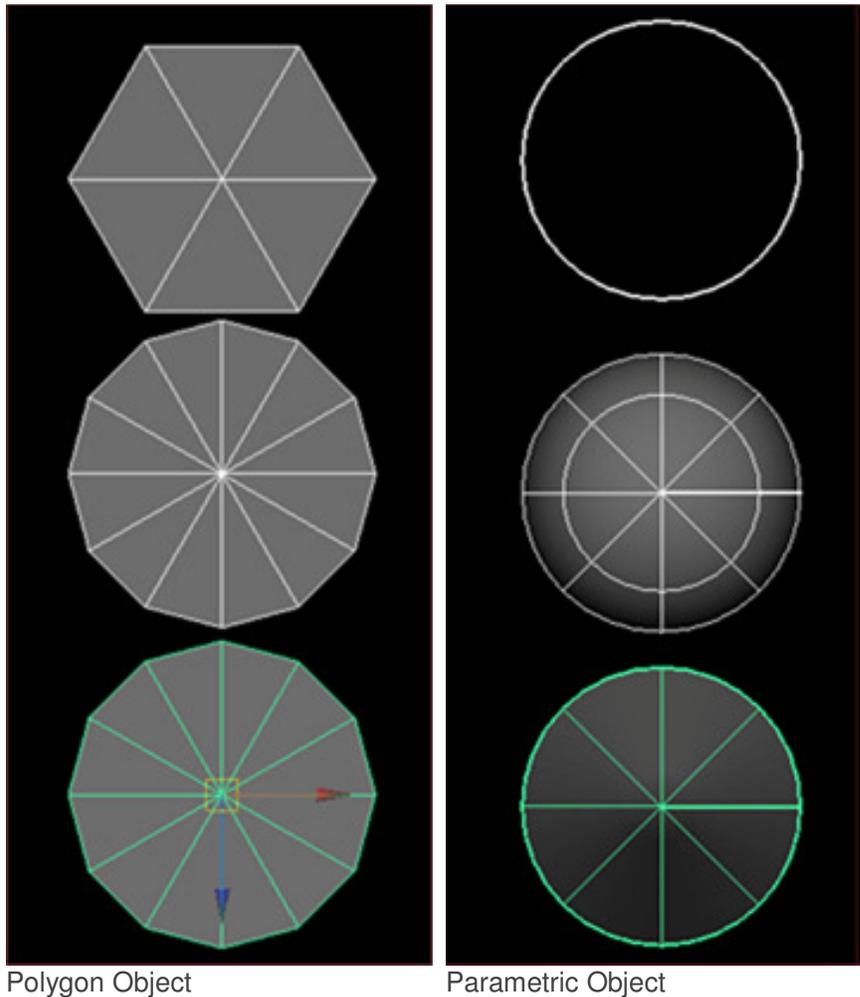
The handling of these two types of geometries is different from a renderer to renderer and it makes a huge difference in time spent for rendering. As for rfm, it can render three main surfaces from Maya, Polygons, NURBS, Subdivision surfaces (a type of polygon object with parametric handlers), during the test renders, it was proved that Renderman renders NURBS surfaces much faster than Mental Ray since it is by nature a parametric renders. That also helps in rendering subdivision surfaces.
